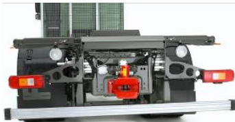
Lighting installation validation (UN Reg 48)
