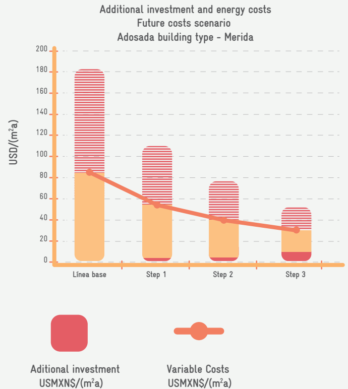
Figure 19: Future costs of the different steps towards the “step by step refurbishment to achieve optimal energy and environmental performance” standard (efficiency improvements) for Adosada building type (50 m² SRE) in Merida (Source: Passivhaus Institut).
